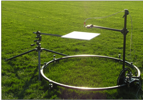
Field goniometer set up over the Lolium perenne field
